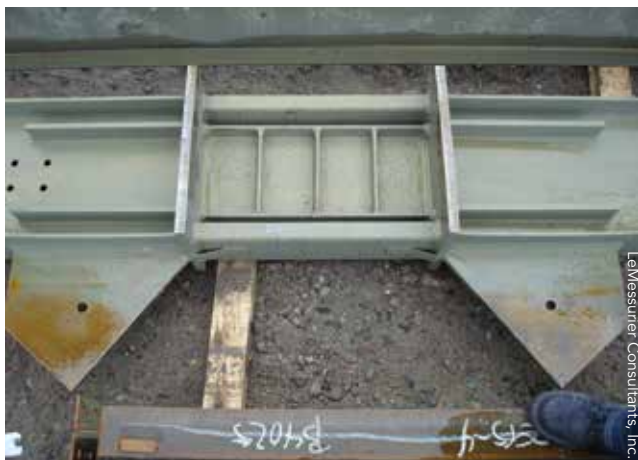
▲ A sample shear link at Dudley Square.
