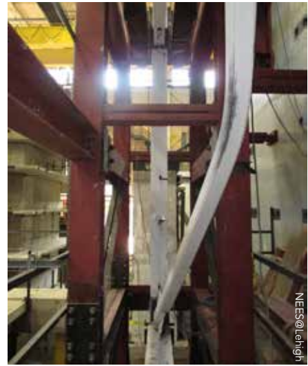
▲ OCBF brace buckling testing.
