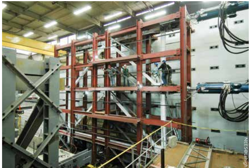
▼ R = 3 chevron braced frame testing.
