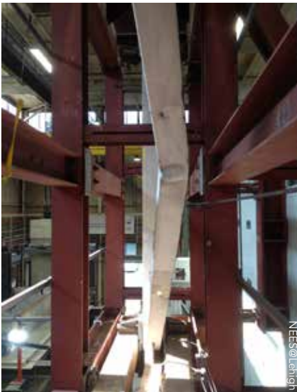
▼ R = 3 brace buckling testing.
