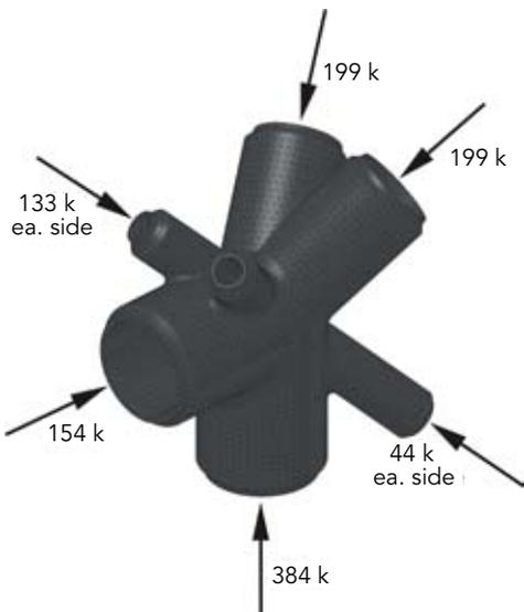
▲ **This page:** The nose pipe, where eight truss elements come together, was one of four castings used to make the WTC modular steel truss frame connections.
