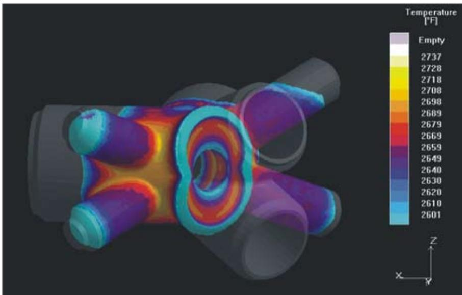
▲ This model of the nose pipe casting was made by the foundry's consultants, Product Development & Analysis LLC, to determine how to arrange the risers and the chills for the cooling process.
